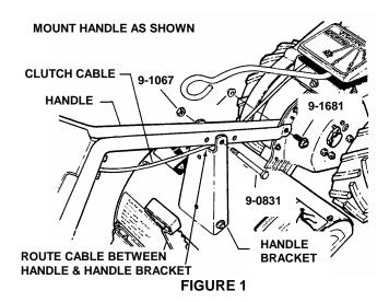
STEP 3: Handle bar adjustment can made by removing Part Number 9-0831, Hex Cap Screw and Part Number 9-1067, Hex Lock Nut from handle bar bracket and handle bar and moving into another hole position. Adjust handle bar "UP" or "DOWN" as required in the corresponding "Low", "Medium", or "High" holes located in the handle bar. See Figure 2.
